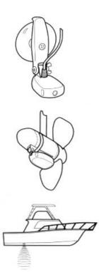
Thru-hull mounting may require the use of a fairing block to level the transducer with the waterline. Also, since special tools and knowledge may be required to perform this type of installation, it is best to refer to a qualified marine technician.
